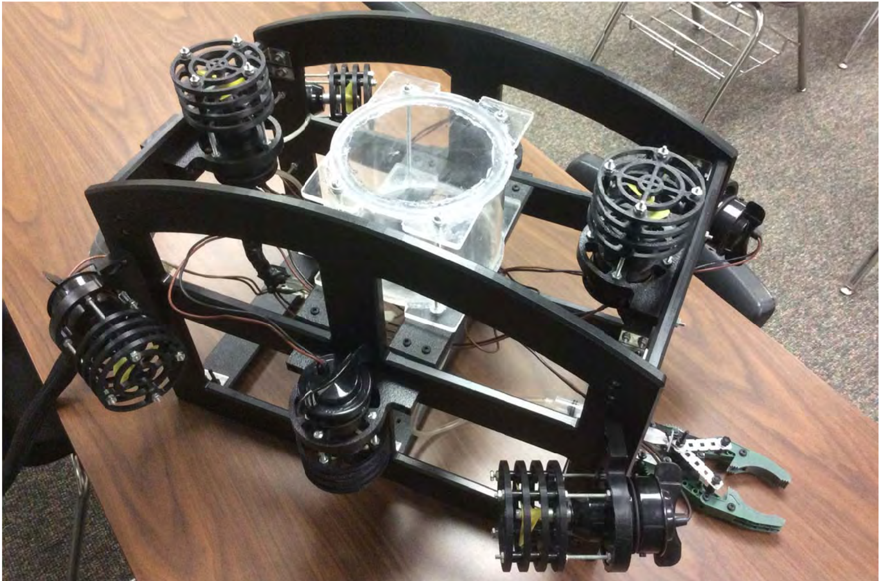
Final version of the ROV. The Attabox has been replaced by a custom acrylic tank for buoyancy. The four horizontal motors are mounted at the corners and angled. The motor mounts have slots cut into them to increase thrust force.
