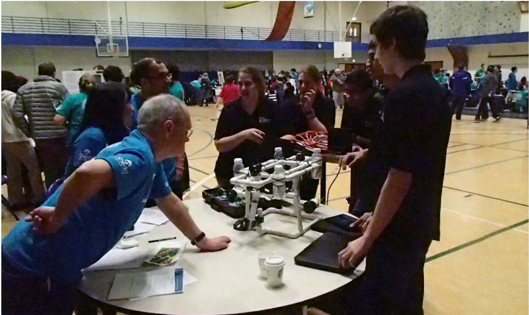
Mock Sales Presentation at the Shedd ROV Club Event. Note the modified frame design – the top is elongated. There are now two vertical motors attached to the top frame at the front and back. Pool noodles have been replaced with plastic bottles. The first version of the claw is attached to the front of the ROV.
