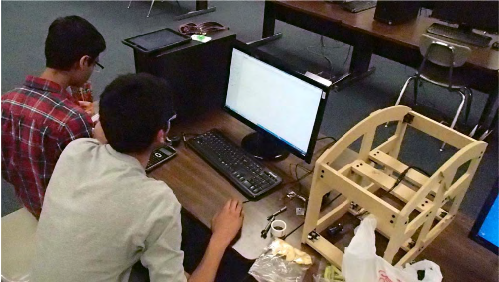
Assembled MDF prototype of new frame design prior to cutting HDPE.
